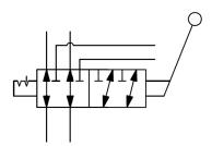
The OP80 Six Port Valve Series is a manually operated spool type 6-way 2-position selector valve. The high-quality cast-iron valve body is cast in Australia machined at Oilpath's Adelaide facility along with the plated hardened steel spools that have a metering facility that a smooth transition when moving between circuits and the other. The range also includes alternative actuation methods.
