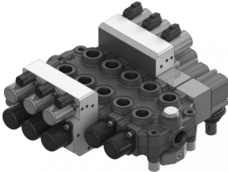
OP20 configured with 3 solenoid actuated spools with manual override and 2 manually operated spools (in the upside-down configuration). Typically utilised in Tilt Tray applications
